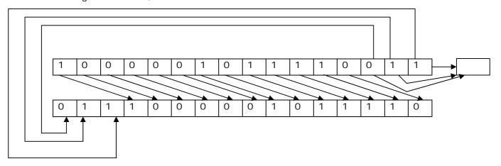
Here rotate by 3 operation is shown. It is clearly seen that every bit is assigned to a new position that is 3 places away from previous one. Unlike the shift command no right bit is destroyed. It is placed in the leftmost position.
